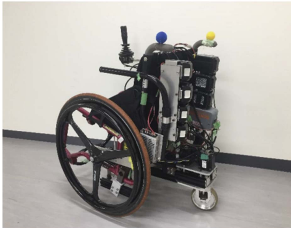
Figure 13: Wheelchair with a differential active caster drive system.
