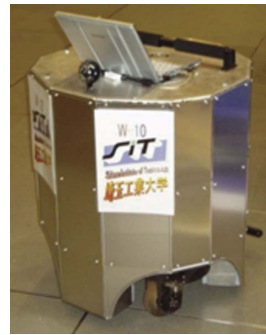
(b) Omnidirectional robot overview
