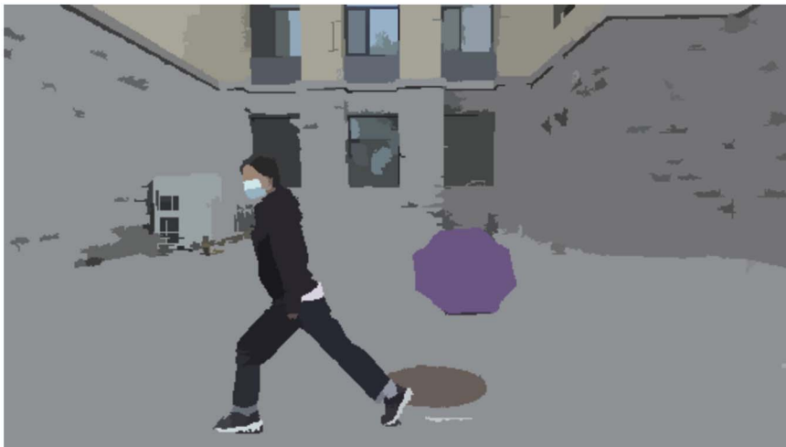
Figure 9: Color image segmentation with Mean shift. (a) original color image; (b) segmentation result.
