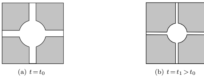
FIG. 2.2. Evolution of the pore. The structure of the node and bond is uniquely determined by the porosity \phi^\varepsilon(x,t) at node x , i.e., the radius of node r_n and the radius of bond r_b are only dependent on \phi^\varepsilon(x,t) .
