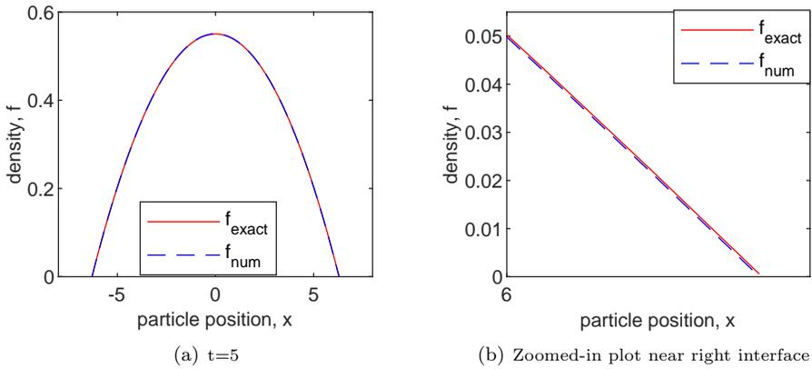
FIG. 8.3. The density  $f$  at time  $t=5$  and zoomed-in plot near right interface with the exact solution  $f_{exact}$  and the numerical solution  $f_{num}$  ( $M=100$ ,  $\Delta t=1/100$ ).
